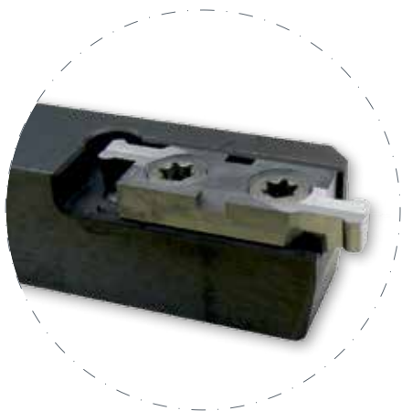
Multi function turning tool with profiled insert
